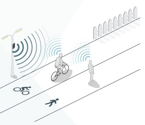
The CityRadar contains a radio transmitter and receiver combined into one unit. The unit emits a low power radio wave and listens for any echo. If there is a cyclist or pedestrian in the path of the radio wave, a part of the radio wave will bounce back. Depending on how long it takes for the signal to return, the radar calculates how far away the object is and in what direction it travels. Based on the profile of the echo, the radar also calculates what type of object that passes in front of it.
