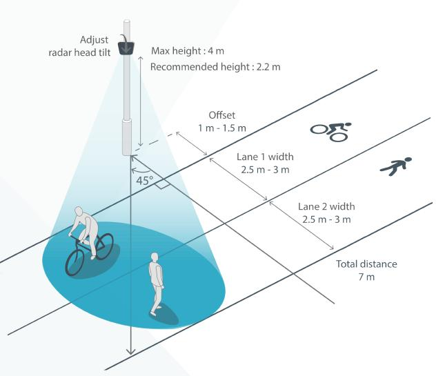
This is a basic description of how to set up and position the CityRadar.
